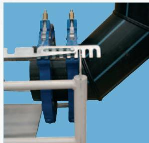
The sliding 3rd clamp provides time saving and a highly flexible system for clamping bends and tees without additional tools. Just take out the spacer block, shift the clamp to the desired position and fix it again with the spacer. A double-sided pulley mechanism enables a secure heater plate separation from the melted pipe ends in all welding positions.
