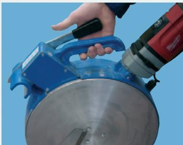
The pipe planer provides improved pipe facing performances thanks to a powerful motor and a re-designed worm-gear torque transmission. Handling of the facing tools is ergonomic thanks to reduced and well balanced weight. User's safety is assured by a spring loaded self-locking mechanism and a micro-switch preventing accidental operation of the motor. Mains cables are wired internally within the housing for full protection against potential damage.
